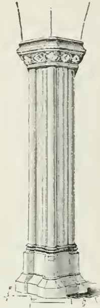
PIER: CLUSTERED PIER OF LATEST TYPE, WITH ONE CAPITAL FOR THE WHOLE. STOGUMBER, CHURCH OF S. MARY, SOMERSET; c. 1500.
